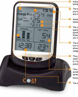
Indicates the number of sensor jaws installed. For most domestic situations this will be one
